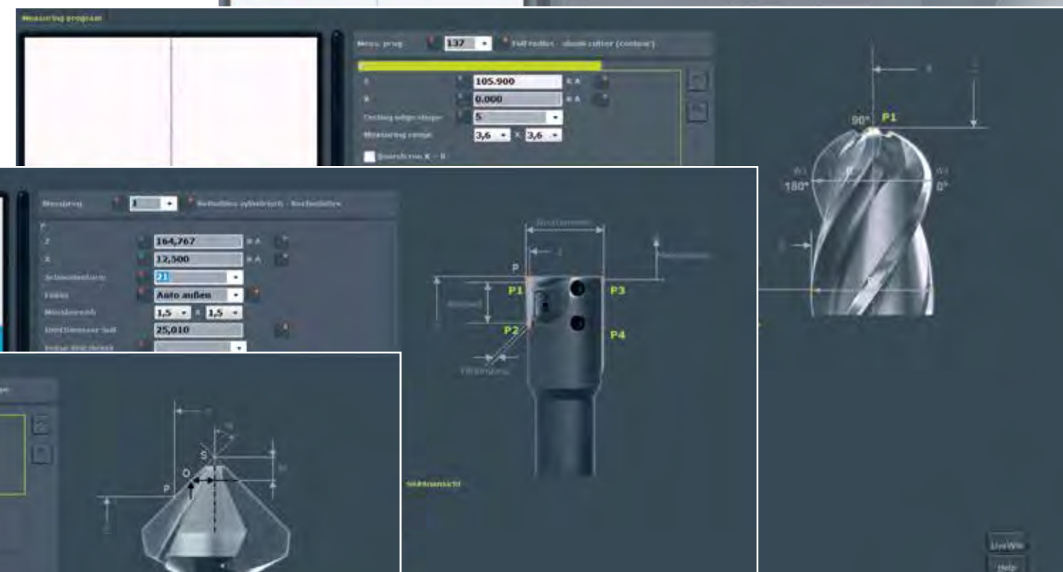
Measuring program 137: For fully automatic determination of the radius contour.
