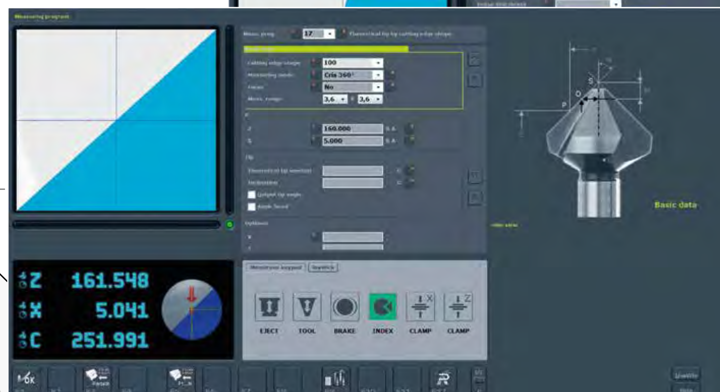
Measuring program 17: To determine the theoretical tip over cutting edge shape.
