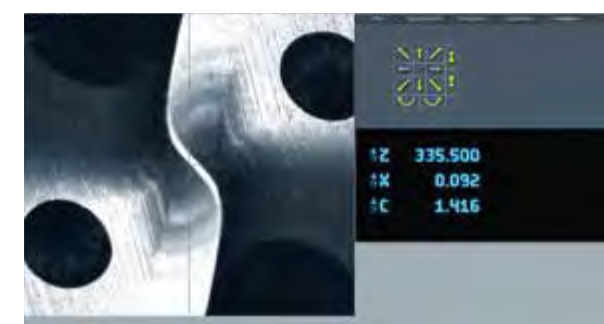
The face of the tool is displayed and measured in the »metis« tool analysis software.
